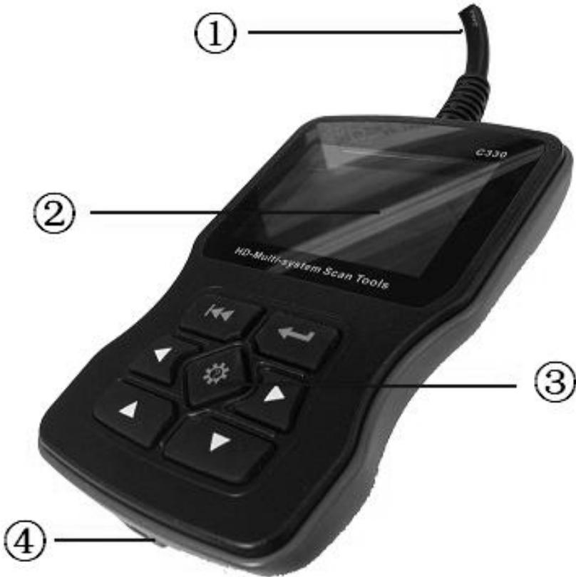
① **DLC** -- Data Link Connector (DLC), Use to connect the scan tool to the vehicle;
